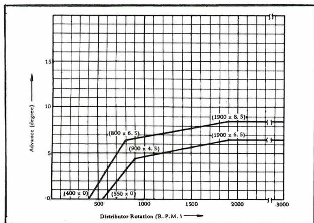
Fig. EE-89 Centrifugal Advance Characteristic
