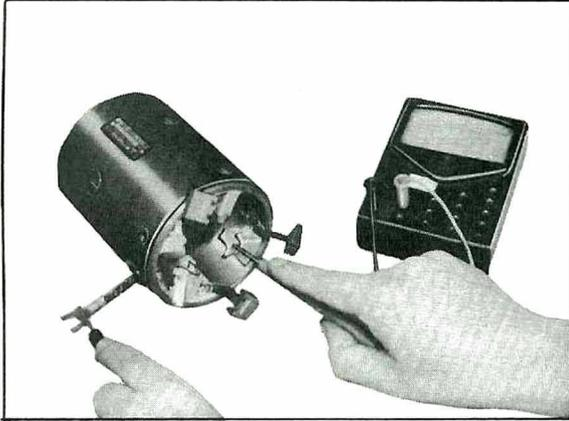
*Fig. EE-58 Field Coil Test for Continuity*
